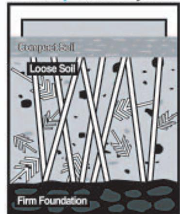
Placement of piles in an EQ-FORCE array reduces seismic shock and it leaves a motion-damping isolation zone directly under the footing. This system converts damaging high frequency shock waves to manageable low frequency effects which can be absorbed by the structure without major damage.
