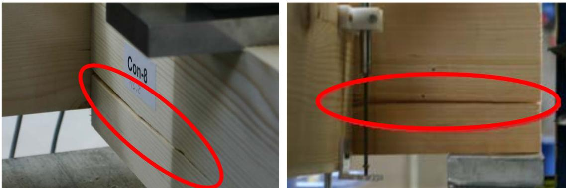
Figure 2 – Brittle failure Rounded Dovetail Joint: joint (left) and main beam (right)
