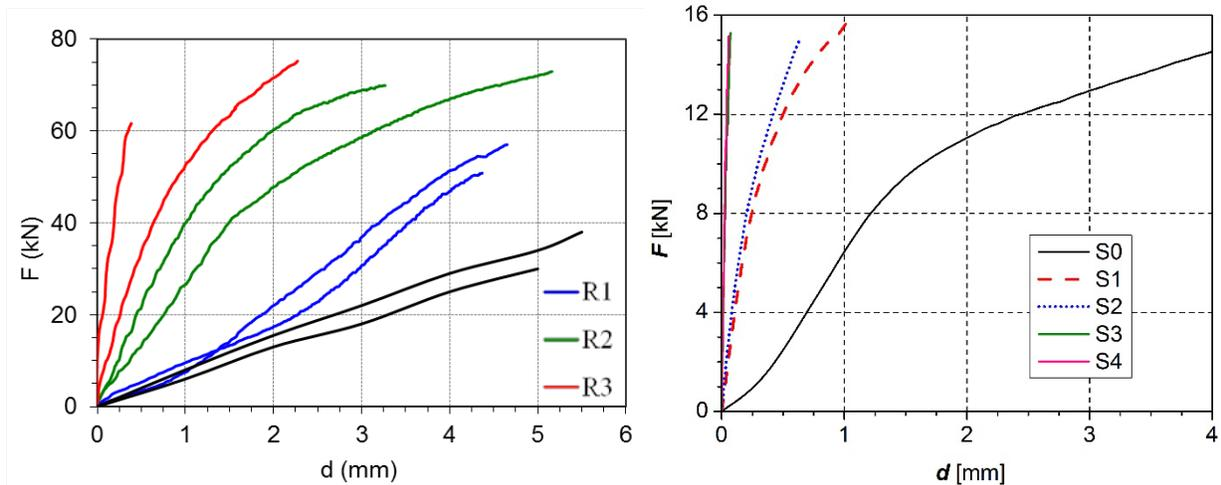
Figure 4 – Load-deformation curves illustrating reinforcement effects
