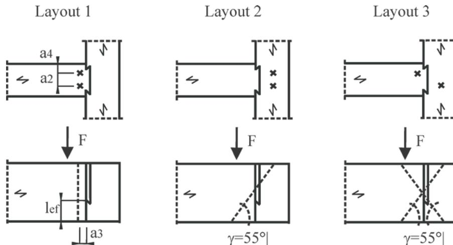
Figure 3 – Layouts of RDJ reinforcements
