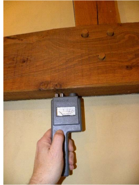
Figure 1 Hand-held resistance-type moisture meter with short pins inserted into the timber measures the MC near the surface of the timber
